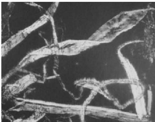
Figure 2.80. The morphology of cellulose fibers. Courtesy of Cellulose Filler Factory Corporation, Chestertown, MD, USA.
